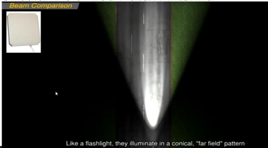
The circular patch antenna projects a far beam in a conical pattern which, when used in dock door portal applications, lends itself to cross-reads and stray reads - reading tags on assets other than those going through that particular doorway.
